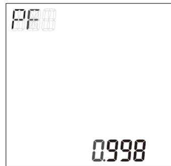
\*Power factor operation is a method assuming balanced load. The error might be big when it measures unbalanced load.
