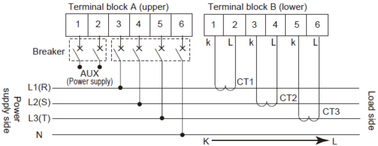
**⚠** Vn terminal should be connected to N-phase which is grounded.
