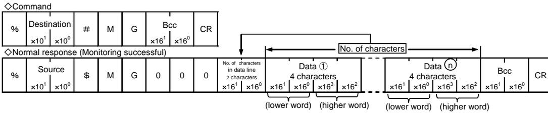
◆[RT]: Read the status of Eco-POWER METER (Reads the specifications of Eco-POWER METER and error codes if an error occurs.)
