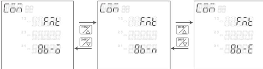
[Set list] 8b-o (8bit odd), 8b-n (8bit none), 8b-E (8bit even) (initial: 8b-o)
