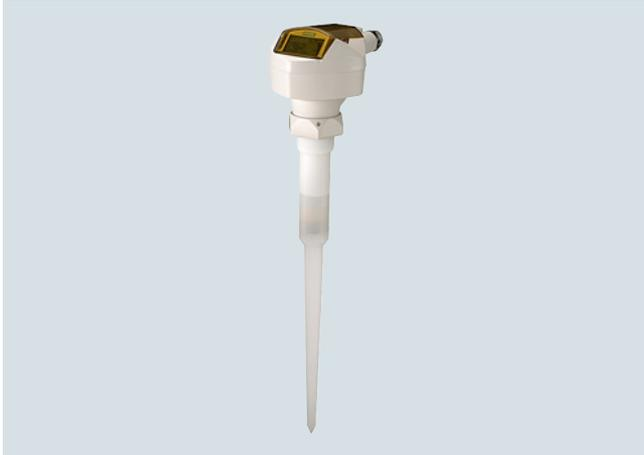
SITRANS Probe LR is a 2-wire, 6 GHz pulse radar level transmitter for continuous monitoring of liquids and slurries in storage vessels with nominal pressure and temperature, to a range of 20 m (66 ft).
