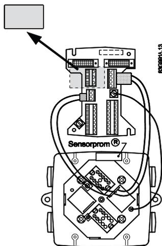
7. Fit supply and output cables through cable glands and connect to connection plate as shown in Electrical connection (Page 36).
