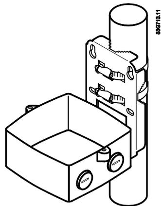
Figure 4-7 Pipe mounting - vertical
