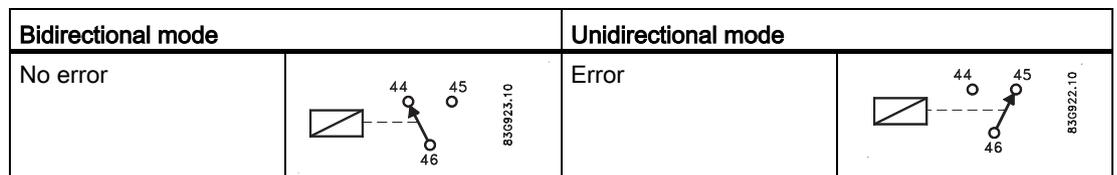
Limit switch (can be used as direction switch)
