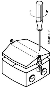
2. Remove SENSORPROM® unit from sensor terminal box and mount it in terminal box of wall mounting unit.
