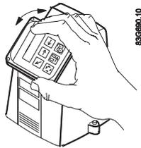
4.6 Turning transmitter/keypad
