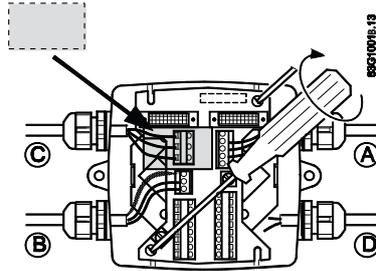
9. Tighten cable glands to obtain optimum sealing.
