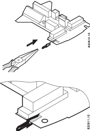
2. Remove hardware key after setting up and calibrating unit.
