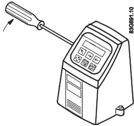
2. Loosen the four screws retaining keypad.
