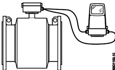
Figure 4-2 Remote installation
