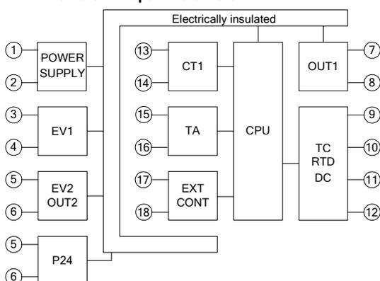
If OUT1 is a non-contact voltage output or direct current output, and if OUT2 is a non-contact voltage output or direct current output, OUT1 is not electrically insulated from OUT2.
