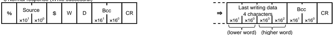
◆[MD]: Register or Reset data monitored (Registers the data to be monitored.) \*Up to 16 points can be registered for one unit.
