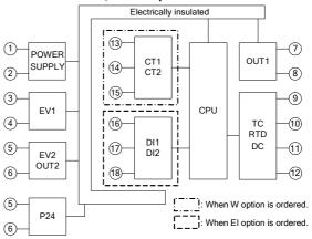
If OUT1 is a non-contact voltage output or direct current output, and if OUT2 is a non-contact voltage output or direct current output, OUT1 is not electrically insulated from OUT2.
