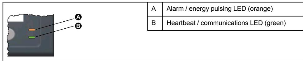
**NOTE:** For the PM5561 model, the alarm / energy pulsing LED is factory set for energy pulsing only and cannot be modified or disabled.
