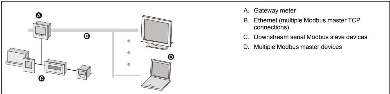
A Modbus master device (such as an energy management system) can communicate through the gateway meter to a serial network of devices connected to the gateway meter’s serial port(s). The meter receives Modbus TCP/IP data on TCP port 502, translates it to Modbus RTU then forwards it to the addressed slave device.
