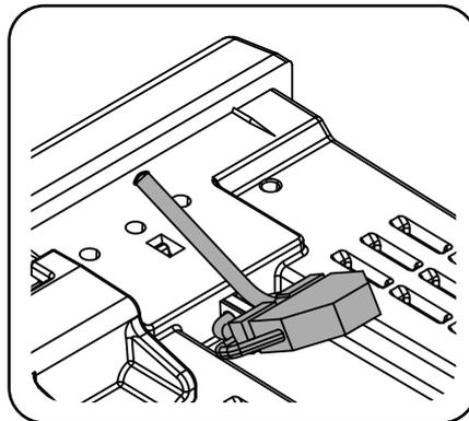
12. Follow the instructions in the installation sheet to Install the meter and apply the anti-tamper voltage and current terminal covers.
