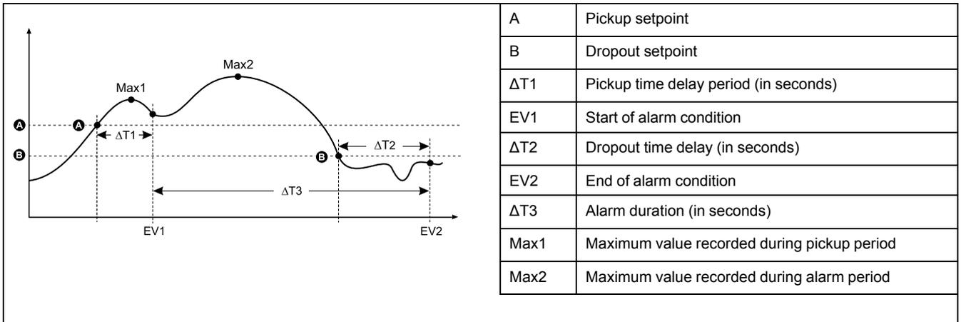
The meter records the date and time when the alarm event starts (EV1) and when it ends (EV2). The meter also performs any task assigned to the event, such as operating a digital output. The meter also records maximum values (Max1, Max2) before, during or after the alarm period.
