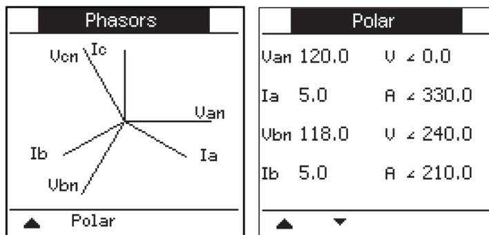
The graph on the Phasors screen shows a representation of the phase angles in degrees. The Polar screen shows the RMS value and phase angle of each voltage and current phases.
