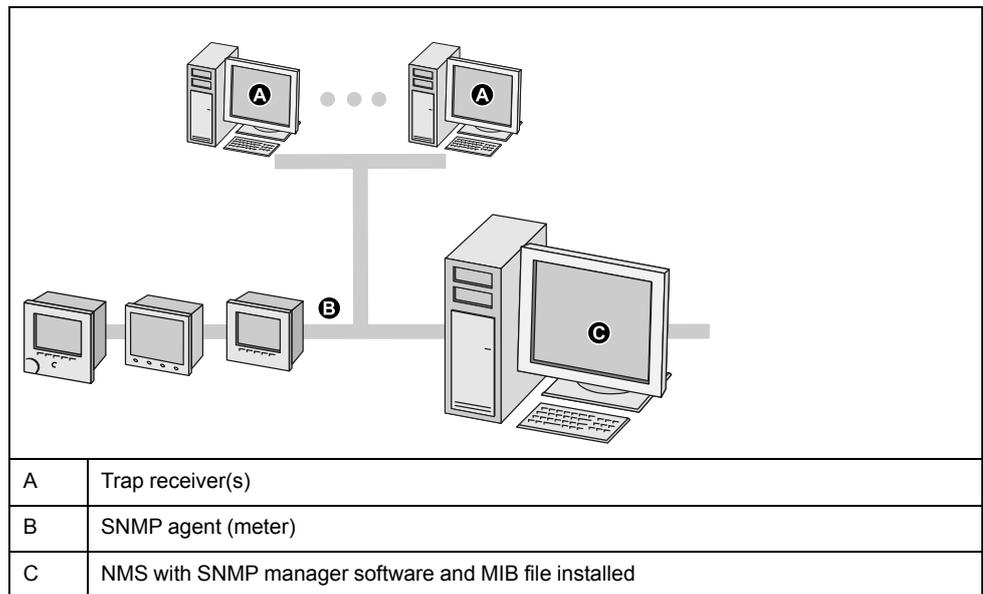
**NOTE:** The NMS computer can also function as a trap receiver.
