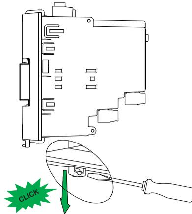
4. Swing the meter out and upwards to remove the meter.
