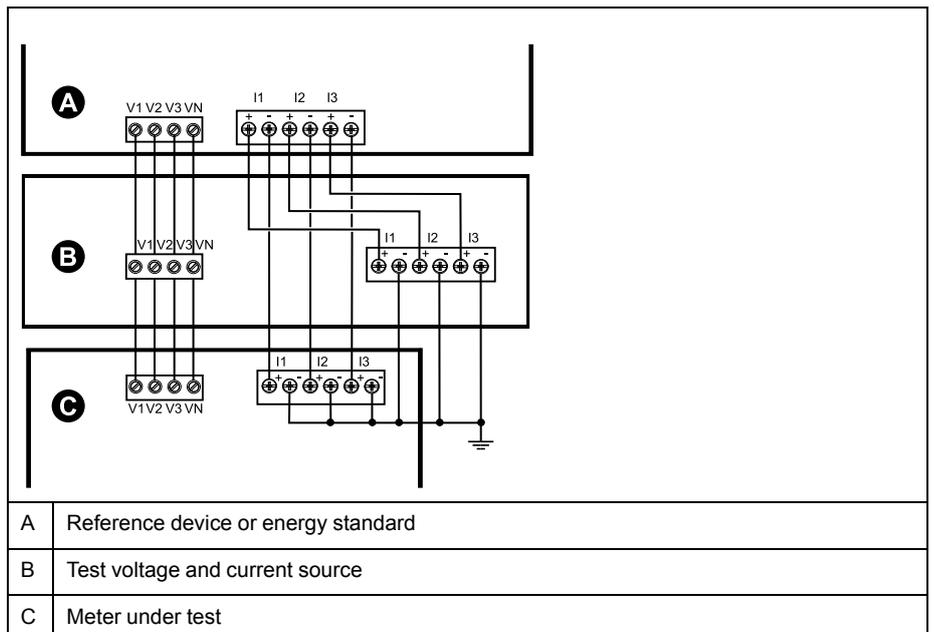
4. Connect the control equipment used for counting the standard output pulses using one of these methods:
